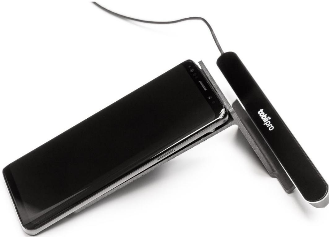
**Figure 5.9** The mobile device and the Pro Nano eye tracker attached to the Sticky Pad on the Device Holder
