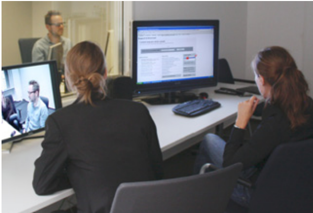
Remote live viewing of eye gaze displayed on the stimulus and user camera.
