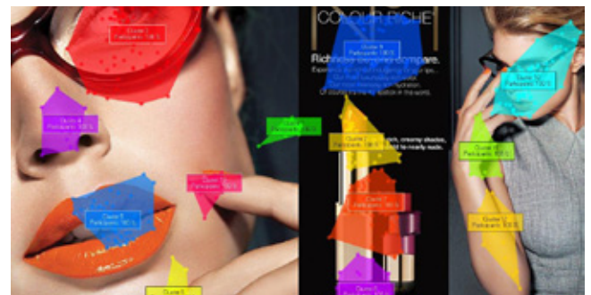
Clusters display areas with a high concentration of gaze points as polygons and can easily be transformed into areas of interest (AOI) for statistical analysis.
