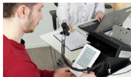
Dedicated solutions allow for testing of mobile devices like tablet PC's or e-readers in natural setups.
