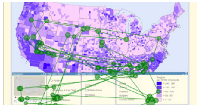
Gaze plots display gaze data from one or several recordings as individual gaze points, fixations and gaze paths. The order and length of fixations can also be visualized.
